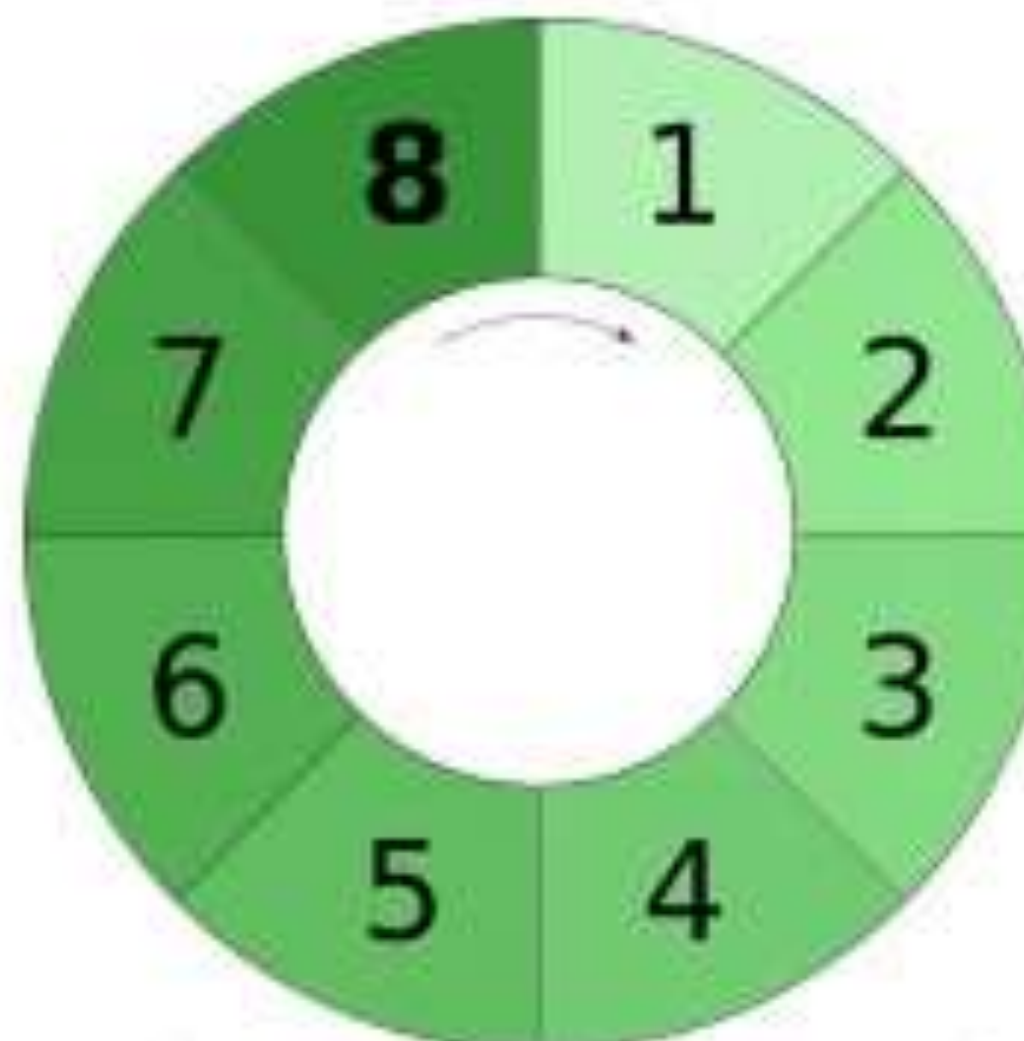
Figure 4 - 8 frames of video recorded into an 8-frame ring buffer.
