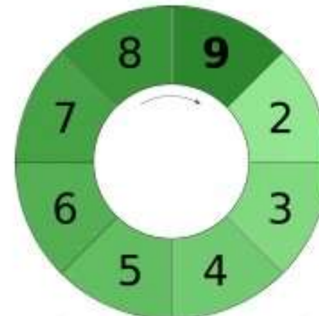
Figure 5 - 9 frames of video recorded. The 9 th frame has replaced the 1 st frame.
