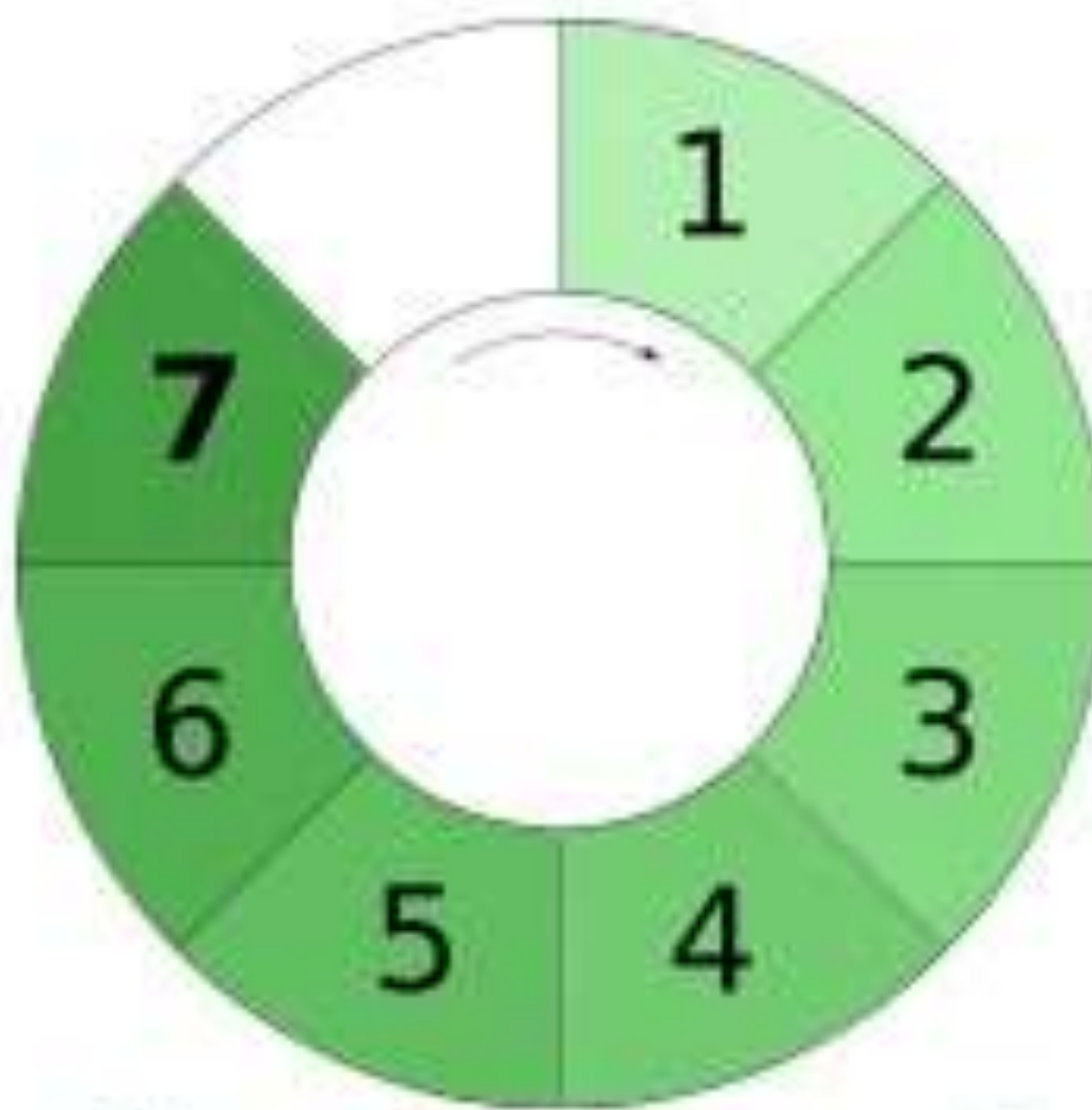
Figure 3 - 7 frames of video recorded into an 8-frame ring buffer.
